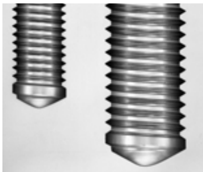
Illustration Sectional view of a thread produced with a drill and thread milling tool.
